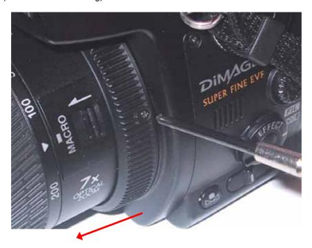
Slide the focus ring towards the rubber part of the lens barrel.
